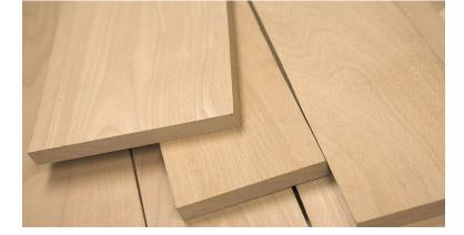
2. Because beech is so stiff, we were able to reduce the thickness of our playfield from 3" to 2.125" to allow for the proper concavity adjustment and playability of the boards while saving weight.
